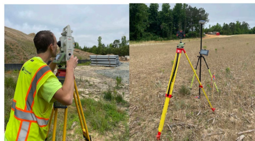
Figure 3: Total station operation (left), Back-sight (right image shown on a yellow tripod), GPS shown on right image as black pole with tablet and round antenna
